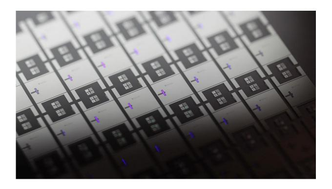
An array of the acoustic wave devices used in the experiment on quantum circuits. The bright purple part is the active part of the device. Credit: Kevin J. Satzinger
