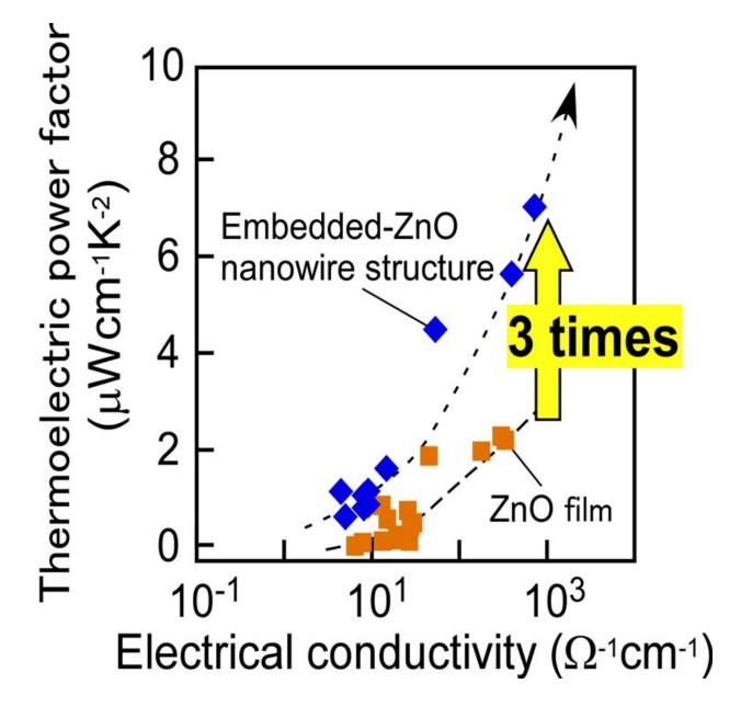
The increase of thermoelectric power factor by introducing nanowires. Embedded-ZnO nanowire structure exhibited a thermoelectric power factor 3 times larger than that of ZnO film without nanowires. Credit: Osaka University
