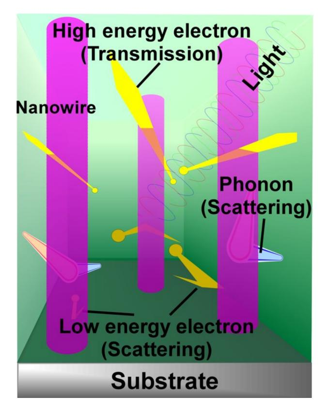
The concept to control electron and phonon transport in Embedded-ZnO
