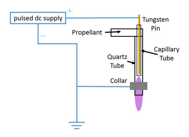
The atmospheric plasma jet can be placed into water to drive a purification process. Credit: Ryan Gott
