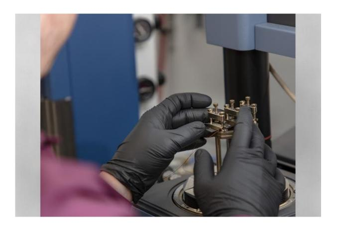
Bowland affixed electrodes on both sides of the cantilever. In a dynamic mechanical analyzer, he clamped one end to hold the beam stationary. The analyzer applied force at the other end to flex the cantilever 100 times. After every 10 flexes, strain was increased, and the electrical resistance was measured as a function of stress to quantify the structural health monitoring sensitivity. Credit: Carlos Jones/Oak Ridge National Laboratory, U.S. Dept. of Energy
