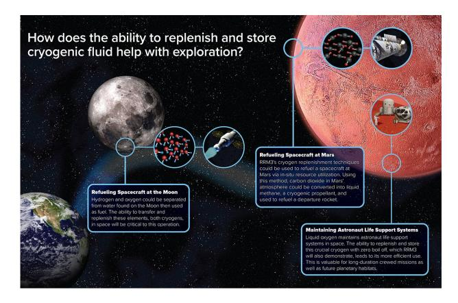
The ability to replenish and store cryogenic fluid can help with exploration. Here are some ways technologies demonstrated by RRM3 could be used at the Moon and Mars. Credit: NASA's Goddard Space Flight Center
