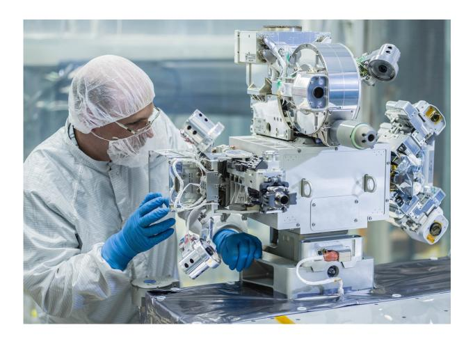
Matt Ashmore, an engineer at NASA's Goddard Space Flight Center in Greenbelt, Maryland, performs a fit check of RRM3's three external tools (from left to right: cryogen servicing tool, VIPIR2, multi-function tool 2). After RRM3 is installed to the outside of International Space Station the Dextre robotic arm will mount the pedestal and tools, pre-assembled by astronauts on the space
