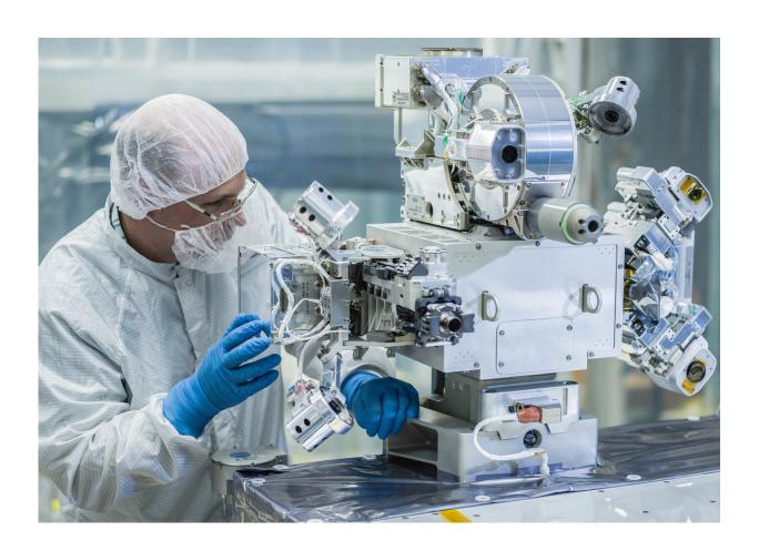
Matt Ashmore, an engineer at NASA's Goddard Space Flight Center in Greenbelt, Maryland, performs a fit check of RRM3's three external tools (from left to right: cryogen servicing tool, VIPIR2, multi-function tool 2). After RRM3 is installed to the outside of International Space Station the Dextre robotic arm will mount the pedestal and tools, pre-assembled by astronauts on the space
