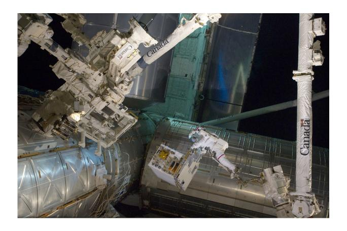
Spacewalking astronauts successfully transfer the RRM module from the Atlantis shuttle cargo bay to a temporary platform on the ISS's Dextre robot for RRM Phase 1 and 2. Credit: NASA
