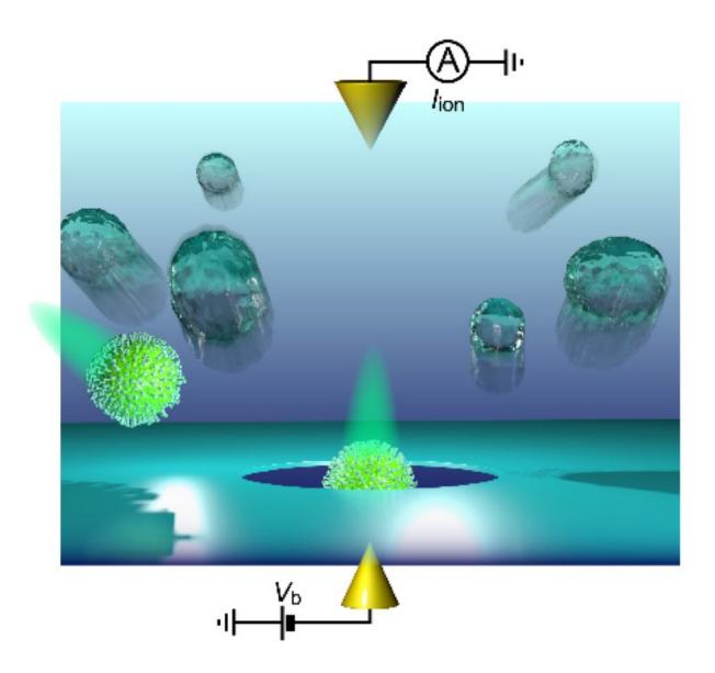
Figure: Detection of a single influenza virion using a solid-state nanopore.
