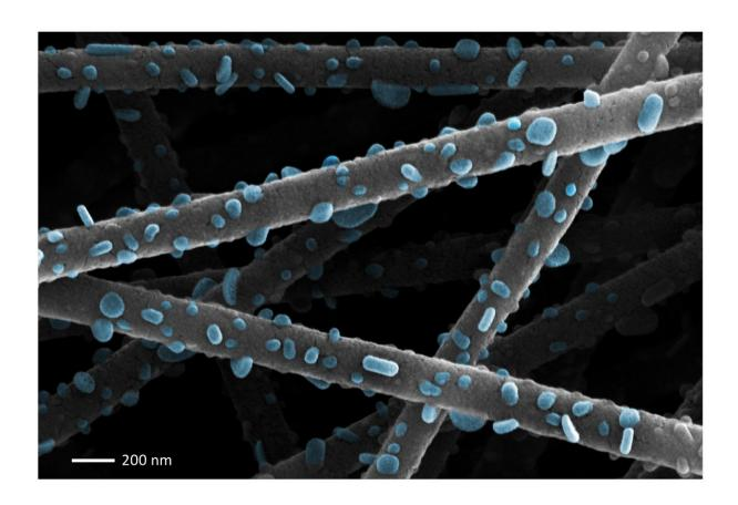
Nanoparticles are visible on the surface of a fuel cell produced by a technology known as electrospinning, which could speed the commercial development of devices, materials and technologies that exploit the physical properties of nanoparticles. Credit: Dr Norbert Radacsi
