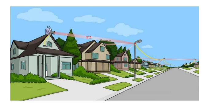
The "last mile" to the internet connection at home is also the most demanding. The new modulator is a viable alternative. In it, data transmitted by millimetre waves (red arrows) can be directly converted into pulses for the optical fibre (yellow). Credit: Salamin Y et al. Nature Photonics 2018
