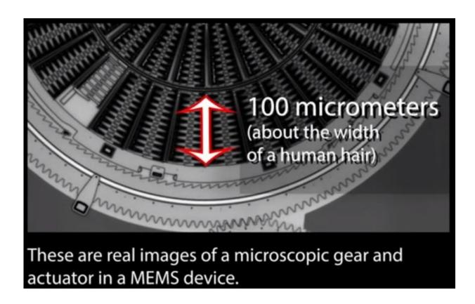
How long can tiny gears and other microscopic moving parts last before they wear out? What are the warning signs that these components are about to fail, which can happen in just a few tenths of a second? Striving to provide clear answers to these questions, researchers at the National
