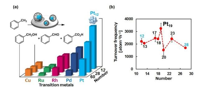
(a) Less oxophilic platinum was superior to other noble metals in the aerobic toluene oxidation. (b) The Pt19 SNC was the highest catalytic performance among other Pt SNCs between 12 and 28 atoms. Credit: *Angewandte Chemie*
