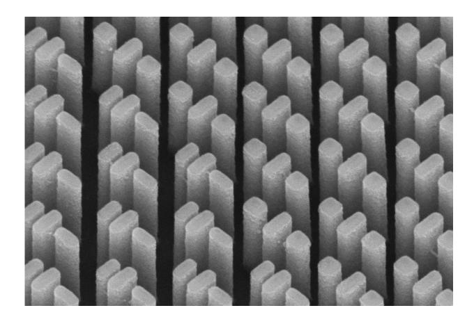
SEM image of the metacorrector. The refractive index of each nanopillar can be tuned and controlled so that all wavelengths are brought to the same focal point. Credit: Harvard SEAS
