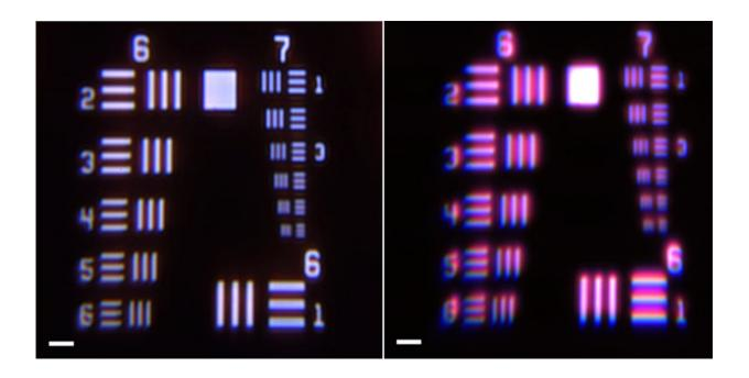
Images of a US Air Force resolution target, a microscopic optical resolution test, imaged with (left) and without (right) the metacorrector. The linewidth of the first line in group 7 of the resolution target is 3.91 micrometers. The scale bar is 25 micrometers. Credit: Capasso Lab/Harvard SEAS
