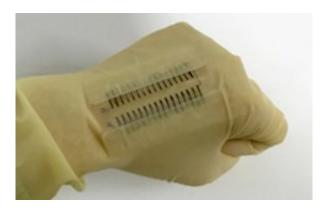
A flexible thermoelectric device embedded in a glove for generating electricity by body heat. Credit: Dr Song Yun Cho, Korea Research Institute of Chemical Technology
