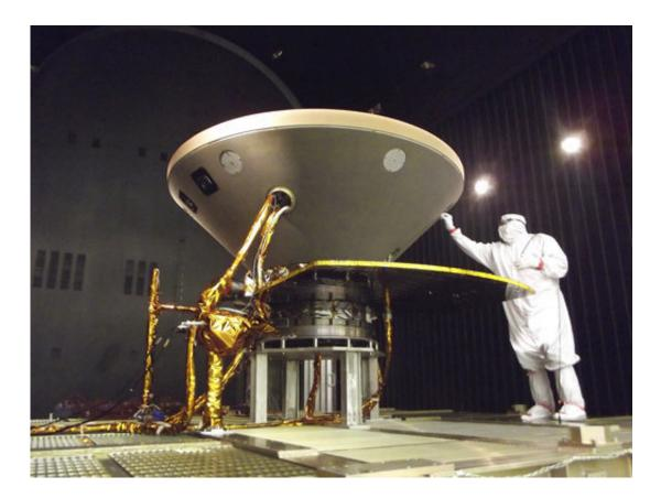
In this 2015 photo made available by NASA, a technician prepares the InSight spacecraft for thermal vacuum testing in its "cruise" configuration for its flight to Mars, simulating the conditions of outer space at Lockheed Martin Space Systems in Denver. NASA's three-legged, one-armed geologist known as InSight makes its grand entrance through the rose-tinted Martian skies on Monday, Nov. 26, 2018. (NASA/JPL-Caltech/Lockheed Martin via AP)
