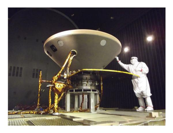
In this 2015 photo made available by NASA, a technician prepares the InSight spacecraft for thermal vacuum testing in its "cruise" configuration for its flight to Mars, simulating the conditions of outer space at Lockheed Martin Space Systems in Denver. NASA's three-legged, one-armed geologist known as InSight makes its grand entrance through the rose-tinted Martian skies on Monday, Nov. 26, 2018. (NASA/JPL-Caltech/Lockheed Martin via AP)
