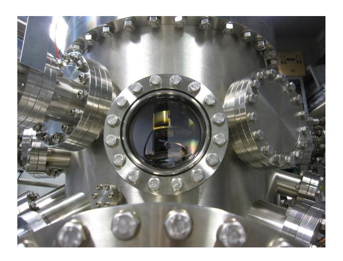
Preparation chamber for alternate catalysts and chemical buffer layers. Picture: Surface Science Group, TU Darmstadt
