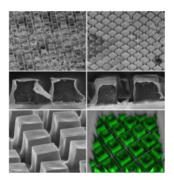
The top and middle rows show microchambers without (left) and with (right) incorporated graphene oxide after dissolution of the templates. The bottom row shows microchambers with graphene oxide after peeling away the template, both scanning electron microscopy (left) and confocal laser scanning microscopy (right) images. Credit: Wiley-VCH Verlag GmbH & Co. KGaA, Weinheim
