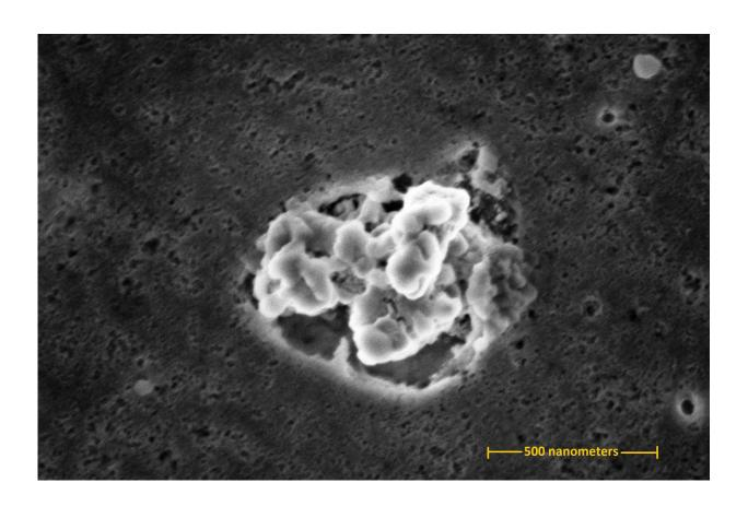
A scanning electron micrograph showing a cluster of silver nanoparticles released by scratching a nanosilver-infused cutting board. The cluster is approximately 900 nanometers across, or about the size of a typical bacterium. Credit: NIST
