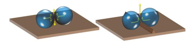
This illustration shows how a ridge architecture and superomniphobic surface causes condensed droplets to jump, rather than coalesce. Credit: Kota Lab/Colorado State University
