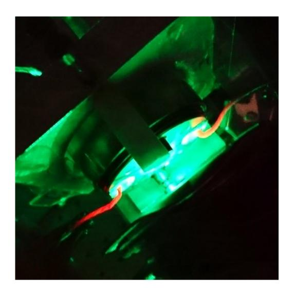
Scientists have recreated an elusive form of nitrogen using a high-pressure diamond-tipped anvil to squeeze tiny amounts of the element at pressures half a million times that of Earth's atmosphere, while heating it to about 500 Celsius. Credit: University of Edinburgh
