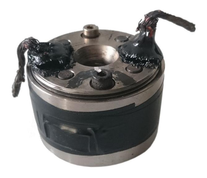
Scientists have recreated an elusive form of nitrogen using a high-pressure diamond-tipped anvil to squeeze tiny amounts of the element at pressures half a million times that of Earth's atmosphere, while heating it to about 500 Celsius. Credit: University of Edinburgh
