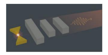
The nanoantenna designed by Ho and co-workers is modeled on the classic roof-top antenna design, but the tiny gold bow-tie shape and silicon dipoles allow it to transmit visible light instead of radio waves. Credit: A\*STAR Institute of Materials Research and Engineering
