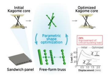
Deconstructing complex shapes into simple mathematical variables has enabled researchers to design and fabricate extremely strong cores for sandwich panels. Credit: Elsevier
