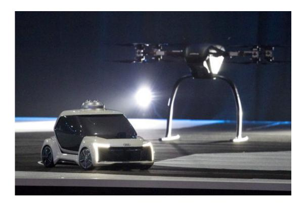
A working scale model of Pop.Up Next, a prototype designed by Audi, Airbus and Italdesign, drives away from the air module, rear, after landing during a presentation at the Amsterdam Drone Week in Amsterdam, Netherlands, Tuesday, Nov. 27, 2018. The two-seater vehicle combines ground transportation with vertical take-off and landing capabilities. (AP Photo/Peter Dejong)
