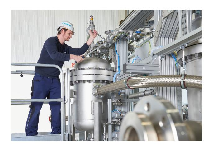
Using a proton exchange membrane electrolyser to produce hydrogen from renewable electricity and water can help industry slash emissions. Credit: Siemens
