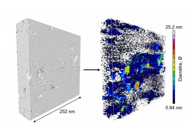
Using a high-resolution system called electron tomography, researchers probed a tiny sample of kerogen to determine its internal structure. At left, the sample as seen from the outside, and at right, the detailed 3-D image of its internal pore structure. Credit: Massachusetts Institute of Technology
