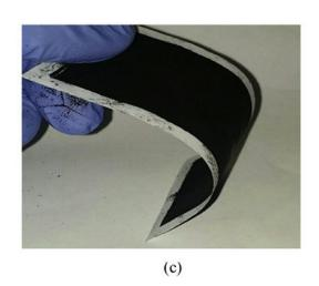
(a) schematic of the symmetric paper supercapacitor with the structure of GNPs electrodes (b) image of the fabricated supercapacitor (c) image of paper supercapacitor in bend state. Credit: *Heliyon* DOI: 10.1016/j.heliyon.2018.e00862
