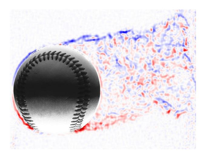
The baseball in this illustration of a knuckleball pitch is moving to the left, leaving a wake trailing behind (i.e., to the right). The blue-colored air is rotating clockwise; the red air is rotating counterclockwise. The drag on the ball depends on the wake size, which depends in turn on the distance between the uppermost blue and lowermost red points. The upward wake means the ball is being pushed downward. Credit: Sakib and Smith
