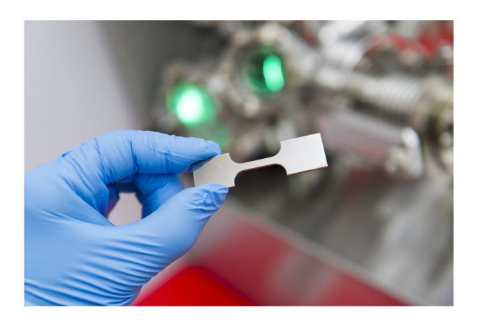
The new alloy Al<sub>7</sub>Ti<sub>7</sub> exhibits a superior strength of 1.5 gigapascals and ductility as high as 50 percent in tension at ambient temperature. Credit: City University of Hong Kong
