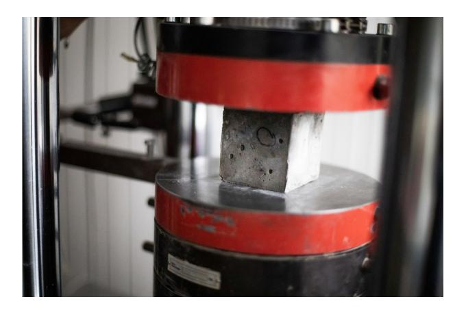
After several years of intensive work KTU scientists succeeded to develop alkali activated concrete, which compressive strength is 55 MPa (the same as in usual concrete). Credit: KTU
