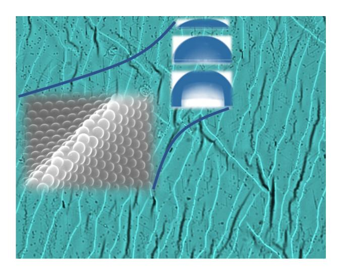
The buckling nature of pre-strained PDMS was applied to the investigation of the dependency of surface hydrophobicity on different geometries of wavy polystyrene thin films, which were fabricated using colloidal self-assembly. This approach can be further applied for fabricating various polymeric nano-films with controlled hydrophobicity. Credit: World Scientific
