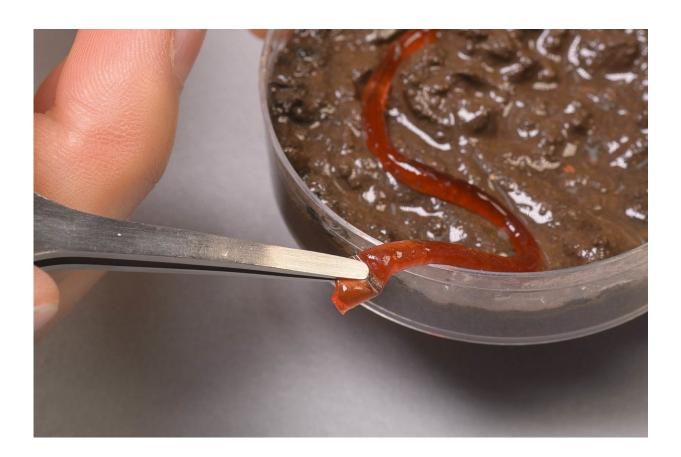
Like the earthworm: The new INM breathing system lubricates itself when pressure is applied to the material. Credit: Iris Maurer
