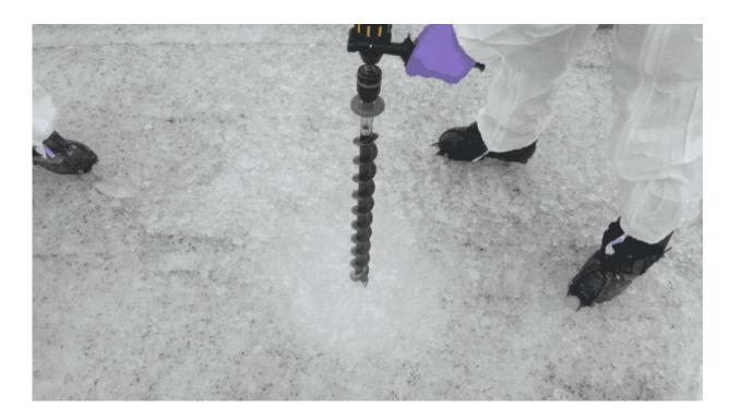
NASA Goddard scientists drill through ice on top of glacier-covered volcano in Iceland to collect samples from deep below. During this summer 2018 research trip, the scientists sought to examine the life forms that could survive in the solar system's harshest environments. Credit: Molly Wasser / NASA Goddard
