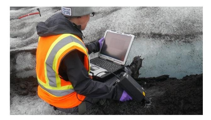
NASA Goddard astrobiologist, Dina Bower, is using a technique called "Raman spectroscopy" to analyze the chemistry of ash-covered ice in a glacier-covered volcanic region in Iceland called Vatnajökull. Credit: Molly Wasser/NASA Goddard Space Flight Center
