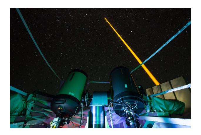
The experiment on La Palma: The laser beam (yellow) generates an artificial guide star in the mesosphere. This light is collected in the receiver telescope (front left). The laser source and the receiver telescope are eight meters away from each other. Credit: Felipe Pedreros Bustos
