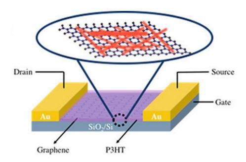
Diagram of the graphene-P3HT nanowire hybrid field-effect transistor. Placing the nanowire mesh (red) on top of the graphene (purple) improves the device's response to light. The silicon dioxide/silicon (grey) substrate, or "gate" electrode, controls the flow of electrical current between the electron source and drain (in this case, Au, or gold, electrodes). The scientists used electron-beam lithography to pattern the device. Credit: Brookhaven National Laboratory
