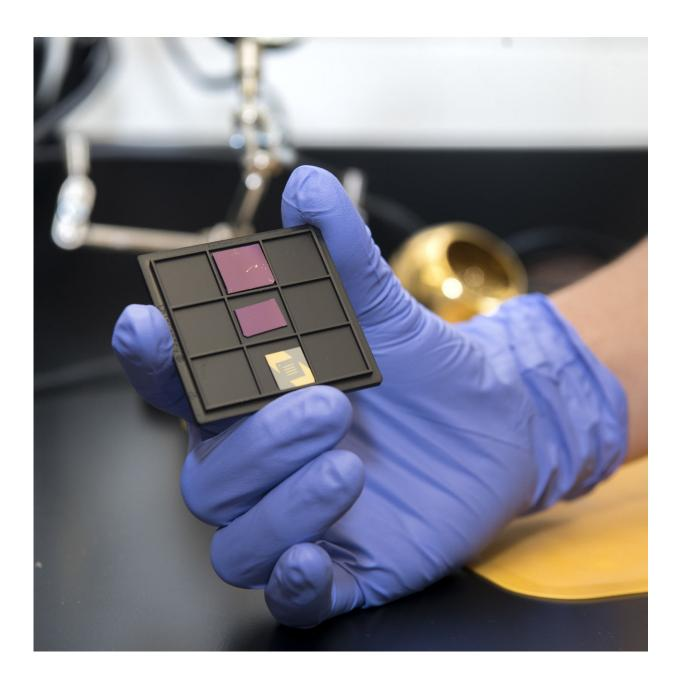
Nanoelectronic devices made from atomically thin materials on a silicon chip.
