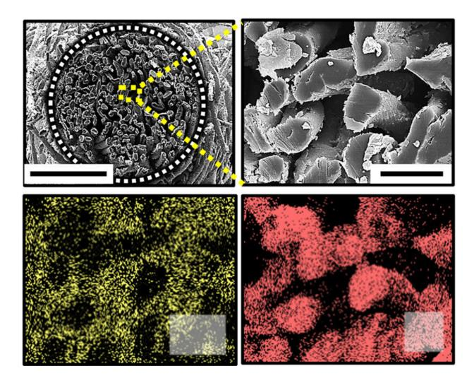
Scanning electron microscope images show details of the cotton-based electrodes used in a new biofuel cell. Credit: Georgia Tech/Korea University
