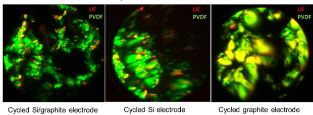
The decomposition of a polyvinylidene fluoride (PVDF) binder in a high energy battery. Credit: Jigang Zhou
