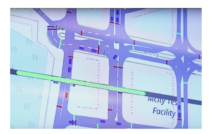
An image of the screen in the Michigan Traffic Lab while a virtual train (in green) travels through a rail crossing at Mcity. Real (red) and simulated vehicles (blue) react. Credit: Screen capture from a video by Mike Wood
