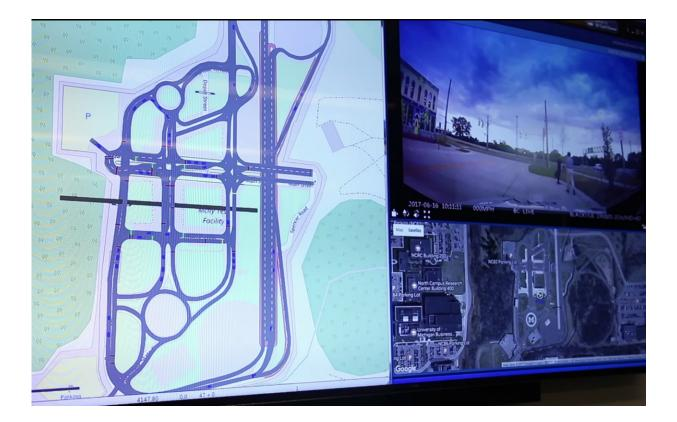
Virtual connected vehicles (blue) can be seen traveling at Mcity alongside real connected and automated vehicles (red). This unique type of augmented reality can dramatically accelerate testing of connected and automated vehicles and enable researchers to test scenarios in a safer, more cost-effective manner. Credit: Screen capture from a video by Mike Wood
