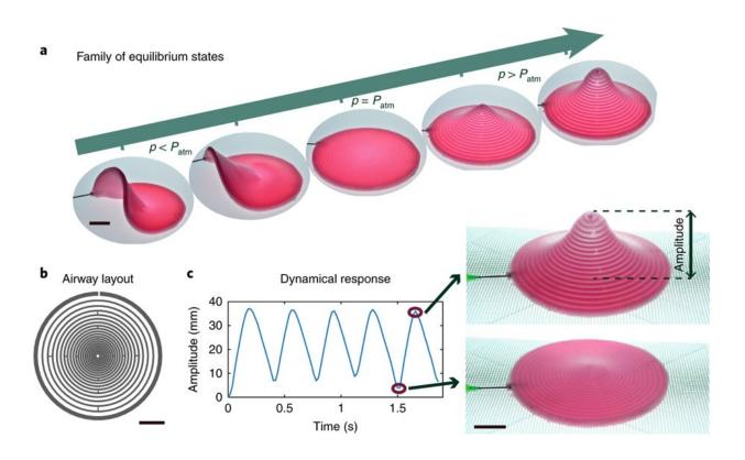
a, Continuous family of equilibrium states obtained for a baromorph under different pressures. b, Corresponding network of channels embedded in the plate. Channels are more concentrated in the central region of the disk, which leads to a spiky structure once inflated. c, Dynamical response: actuation at approximately 3 Hz of the pneumatic system (Supplementary Video 6). Scale bars, 2 cm. Credit: *Nature Materials* (2018). DOI: 10.1038/s41563-018-0219-x
