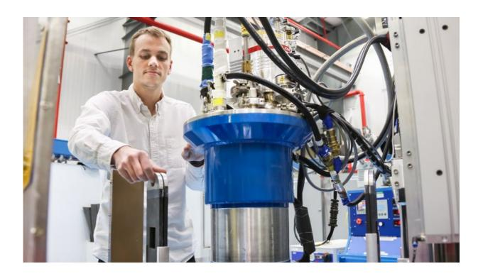
Tyson Lanigan-Atkins, a PhD student at Duke University, uses the cold (lowerenergy) neutron triple-axis spectrometer at ORNL's High Flux Isotope Reactor to study thermoelectric materials. Credit: ORNL/Genevieve Martin
