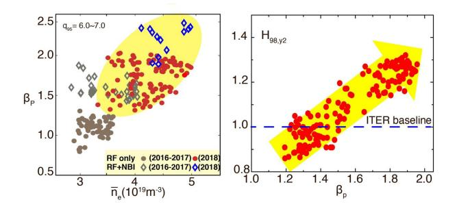
The extension of EAST operation scenario in 2018, with the comparion of its energy confinement enhanced factor to the ITER baseline scenario. Credit: EAST Team
