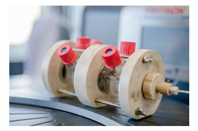
The researchers carried out the experiments in this electrolysis cell. Credit: RUB, Marquard
