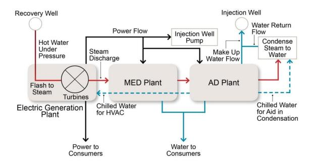
Diagram of how the geothermal energy would be used for energy production, and two types of desalination (MED and AD). Red lines indicate hot water, while blue lines are cooled water. At the end of the process, distilled water would be available for consumers and aquifer storage, and the chilled water could be used in air conditioning for the plant. The whole theoretical system is carbon-neutral. Credit: Courtesy of Thomas Missimer. Credit: Geological Society of America
