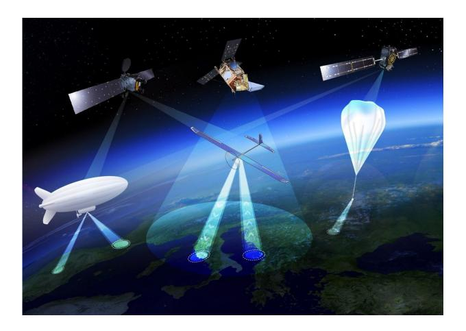
High Altitude Pseudo-Satellites, or HAPS, are platforms that float or fly at high altitude like conventional aircraft but operate more like satellites – except that rather than working from space they can remain in position inside the atmosphere for weeks or even months, variously enabling precise monitoring and surveillance, high-bandwidth communications or back up to existing satellite navigation services. Credit: ESA Earth Observation Graphics Bureau
