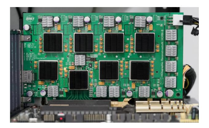
HORN-8 has eight chips mounted on a Field Programmable Gate Array (FPGA) board. Credit: Tomoyoshi Ito
