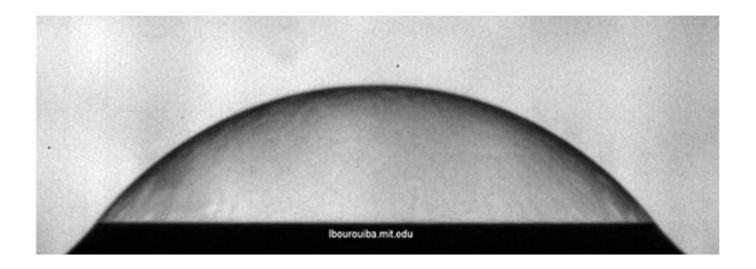
When an old bubble bursts at the water surface, its cap fragments into numerous small droplets. Credit: Massachusetts Institute of Technology
