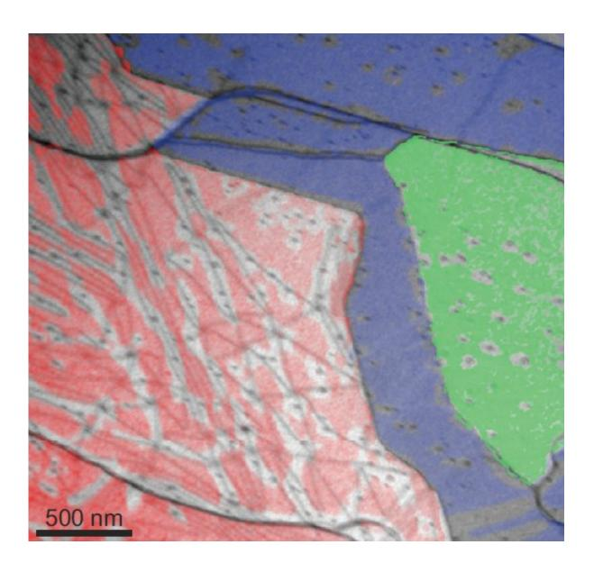
LEEM image of a graphene layer grown on a silicon carbide substrate. A red color indicates the presence of hydrogen atoms sandwiched between graphene
