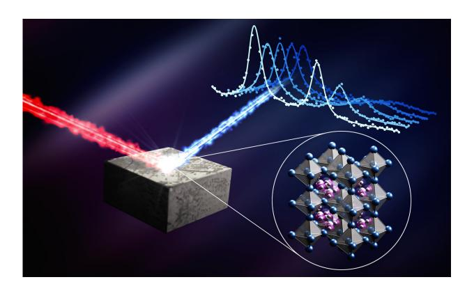
When the researchers scattered neutrons off the perovskite material (red beam) they were able to measure the energy the neutrons lost or gained (white and blue lines). Using this information, they were able to see the structure and motion of the atoms and molecules within the material (arrangement of blue and purple spheres). Credit: Greg Stewart/SLAC National Accelerator Laboratory
