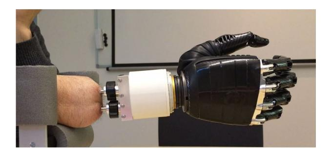
An implant is placed into each of the two bones of the forearm -- the ulna and radius -- and then a wrist-like artificial joint acts as an interface between these two implants and the prosthetic hand. Credit: Biomechatronics and Neurorehabilitation Laboratory/Chalmers University of Technology
