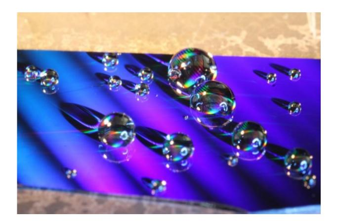
This photo shows water droplets placed on the nanostructured surface developed by MIT researchers. The colors are caused by diffraction of visible light from the tiny structures on the surface, ridges with a specially designed shape. Credit: Kyle Wilke
