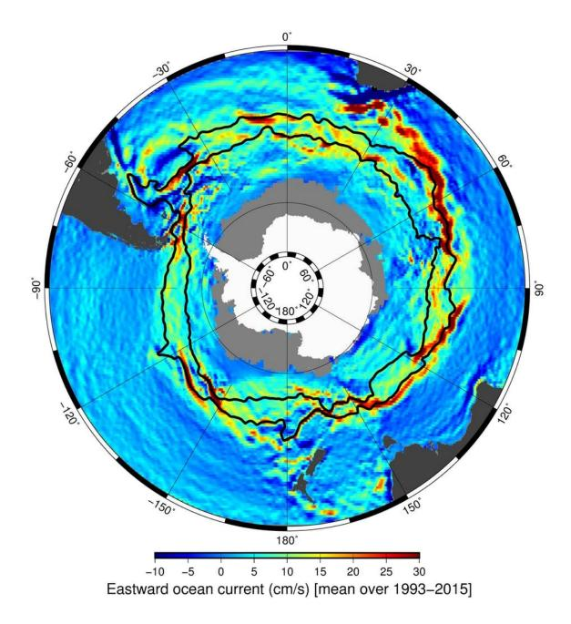
Map of how fast the waters around Antarctica are moving in an easterly direction. It is produced using 23 years of satellite altimetry (ocean height) observations as provided by the European Copernicus Marine Services. Author provided
