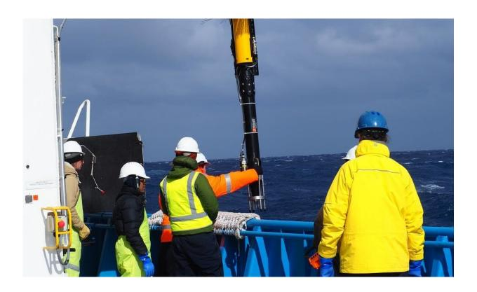
Scientists deploying a vertical microstructure profiler (VMP-2000), which measures temperature, salinity, pressure and turbulence, from RV Investigator in the Antarctic Circumpolar Current, November 2018. Credit: Nathan Bindoff
