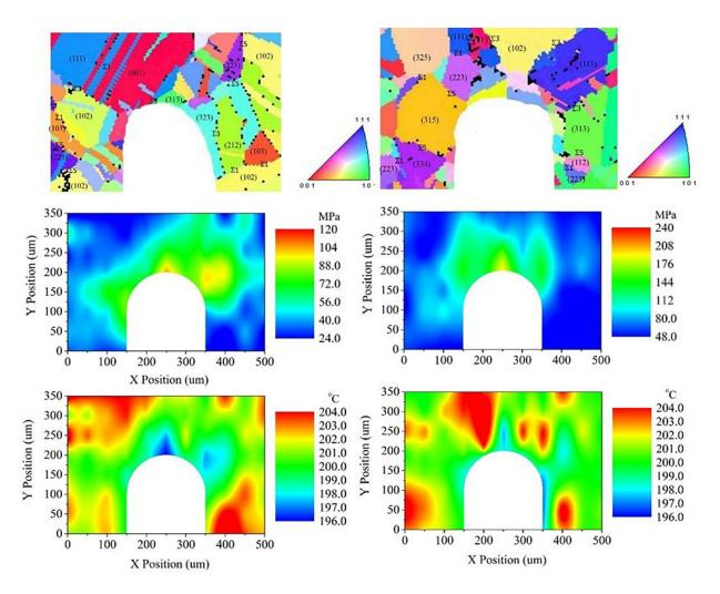
NMRS Measurements of Stress and Temperature Fields in a Superalloy
